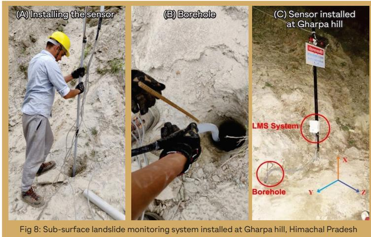
Fig 8: Sub-surface landslide monitoring system installed at Gharpa hill, Himachal Pradesh
